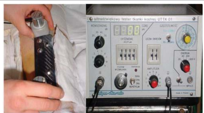
Figure 10: Ultrasonometer tests to assess the propagation of ultrasound wave through the fresh bone callus.
