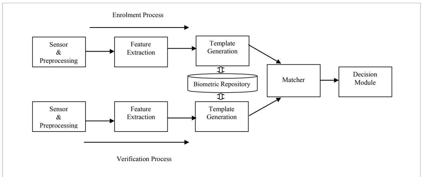
**Figure 1:** Generic biometric processing modes and stages.
