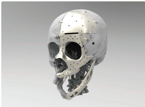
Figure 1D: Computer Assisted Design (CAD) of the facial implant.
