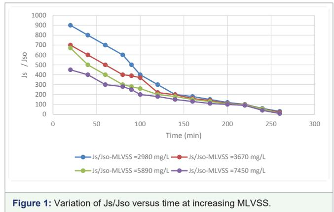
Figure 1: Variation of Js/Jso versus time at increasing MLVSS.
