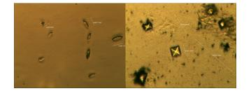
MMS2 treatment showed several oval GOs of 120 micrometer length. (Left: x 250). GNP + Foipan treatment showed several enlarged secondary structures of square GOs of 110 micrometers and partially melted GO remnants of 404 micrometers and of 740 micrometers in length. (Right: x 250). Black clouds in the pictures seem to be Foipan particles.
