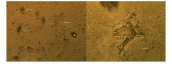
MMS2 treatment showed many partially melted islands of GOs of 110 micrometers and of 120 micrometers (Left: x 250). GNP + Foipan treatment showed a large partially melted-secondary-structures of GOs of 650 micrometers (Right: x 250).
