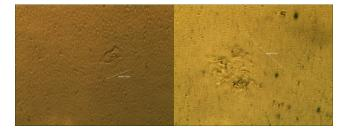
MMS2 treatment showed almost clear background with a 243 micrometer-sized cellular debris. (Left: x 250). GNP + Foipan treatment showed a melted-secondary-structures of GOs of 535 micrometers (Right: x 250). Black clouds in the pictures seem to be Foipan particles.
