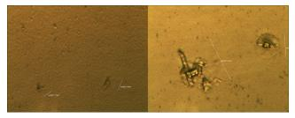
MMS2 treatment showed almost clear background with two melted GOs of 138 micrometers and of 117 micrometers. (Left: x
