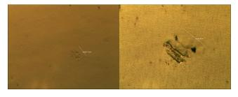
MMS2 treatment showed almost clear background with a melted small remnant of GO of 172 micrometers. (Left: x 250). GNP + Foipan treatment showed partially melted secondary GOs of 393 micrometers on a relatively clear background. (Right: x 250). Black clouds in the pictures seem to be Foipan particles.
