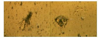
MMS2 treatment showed a melted GO of 701 micrometers. (Left: x 250). GNP + Foipan treatment showed melted GOs of 425 micrometers, 314 micrometers, and a 208 micrometer-sized secondary GO formation. (Right: x 250). Black clouds in the pictures seem to be Foipan particles.
